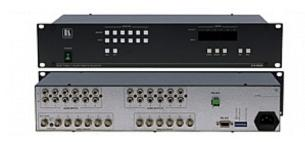
The VS-626 is a high-performance matrix switcher for composite video and unbalanced stereo audio signals. Switching during the vertical interval ensures glitch-free switching with genlocked sources.
