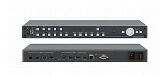
The VSM-4x4HFS is a seamless matrix switcher that can also be used as a 2x2 video wall driver or dual and quad multi-viewers. The unit allows switching between inputs with a clean video cut (frame-to-frame switching with no glitches). The VSM-4x4HFS supports HDMI resolutions with deep color, up to eight channels of audio and includes per-port HDCP and EDID settings.
