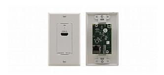
The WP-571 is a DGKat™ wall plate transmitter for HDMI signals. The WP-571 converts an HDMI signal to a DGKat™ twisted pair signal that it transmits to a WP-572.
