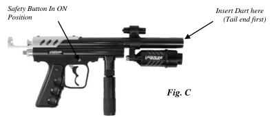
Once the Dart has been loaded into the barrel and you are ready to install your pull line (be sure safety is in the ON position) Pull back on the cocking knob until it locks into place, you are now ready to launce your Dart and install your pull line.
