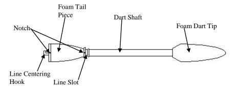
NOTE: line must be attached to the Dart for proper flight stabilization. Therefore, you will need to use the line every time you launch the pull line Dart. Even when sighting in your Laser.
