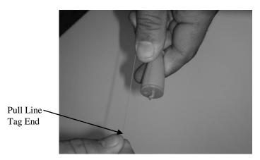
1) Holding the Dart in one hand and the tag end of the Pull Line in the other hand as shown above.
