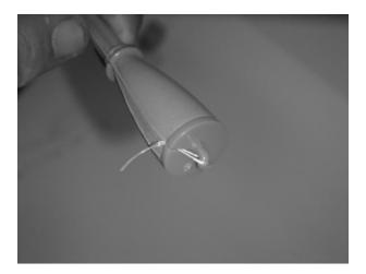
8) Before you insert the Dart into the *LaserLine* barrel, you will need to pull the line back through the notch at the top of the Darts foam tail piece and down through the notch at the base of the Darts foam tail piece. This will secure the line and keep it from dragging in the barrel when launching the pull line Dart.
