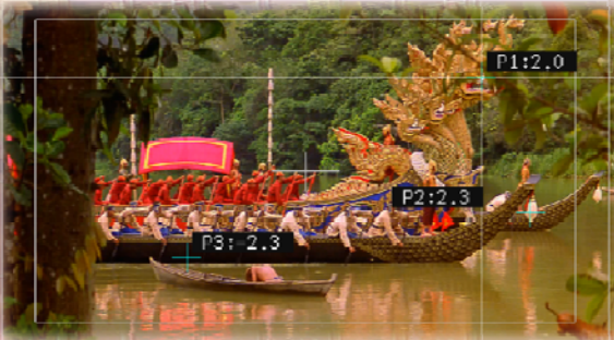
CINELITE "On-Picture" measurements display permits spot measurements in R,G,B, Y% as well as f-stops.
