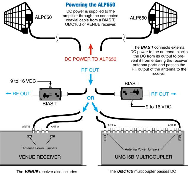
The **VENUE** receiver also includes a DC power pass-through to operate the ALP650 antenna amplifier. Jumpers on the circuit board enable and disable the DC power. The **UMC16B** multicoupler passes DC power from its supply to the antenna input ports to power the ALP650 through the coaxial cable. Jumpers on the circuit board enable or disable the DC power.
