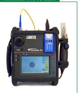
The VC-8200 is an integrated system for fiberoptic connector inspection, evaluation, documentation and cleaning. With built in Wi-Fi, ViewConn Pro can send its Pass/Fail analysis reports via email to other locations or store them directly within the unit. An optical power meter can also be integrated with the unit.
