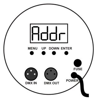
Push MENU to access the operating options. Then use UP and DOWN to scroll through the available choices. When you reach the option you want to set or change push ENTER. Now you can view the current setting for the option and change it using UP and DOWN. Push ENTER to save your changes. The diagram MENU NAVIGATION gives more details.
