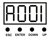
Use UP and DOWN to scroll the available choices. Push ENTER when you reach the option you want to check or set. The current setting for the option will be shown. Use UP and DOWN to change the setting. Push ENTER to invoke the new setting. Use ESC to exit from the sub menus.
