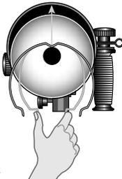
**Warning:** Never operate light without protective screen installed.
