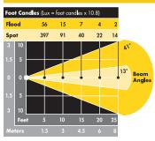
Voltage: 24 V Wattage: 22.4 W Amperage: .7 A Beam control: Continuously variable Fits on: 5/8 stand studs, also 1/4-20 Pistol Grip mount Materials: Primarily aluminum steel. & glass-filled nylon Dimming Control & Switch: in-unit
