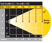
Beam Angles: Points at which intensity drops to 50% of maximum.
