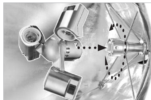
Push in and twist lamphead, locking light fixture base side pins to J-hook cutout. Install flo lamps carefully by holding lamp base.
