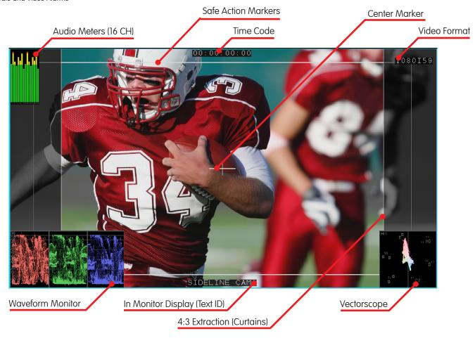
Note: The above screen capture is from a full screen image and shows all of the possible screen overlays. Some can be configured in terms of size and screen position. The video and audio alarms are not shown, and will appear as text on the screen when an alarm condition is triagered. [Video alarms will trigger on "Black" and "No Signal" (video missing). Audio Alarms will trigger on "Silence" and "No Signal" Audio Missing]
