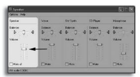
**6.** To adjust the volume of the microphone signal directly to the headphones adjust the **Microphone** fader up or down (this does not effect the volume of the microphone signal being recorded).
