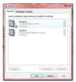
4. To make adjustments to the playback sample rate and bit depth double-click on the speaker icon labeled MXL STUDIO 24 USB. Then click on the tab labeled Advanced. From the drop-down menu, you can change the sample rate and bit-depth for audio playback. When you are finished making changes, click the OK button. \*Please note that you should verify that these settings match the settings in your recording application.
