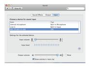
4. Next, click on the **Output** tab and select the device named **MXL STUDIO 24 USB**. You will notice there are no output volume controls for this device. To make adjustments to the volume and other advanced features use the included Studio Control GUI (See page xx for details on the Studio Control GUI). The output volume can also be adjusted in the recording software you are using.
