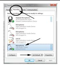
4. To make further adjustments to the recording settings, double-click on the microphone icon labeled **USB Audio Device**. Click on the tab labeled **Advanced**. From the drop-down menu you can change the sample rate and bit-depth for audio recording. Please note that you should verify that these settings match the settings in your recording application.
