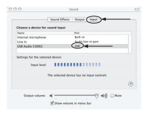
7. By watching the movements of the **Input** level meter in this window, you can now see that the MXL USB microphone is working as you speak into it. This setting will be saved as the default input whenever the microphone is plugged in.
