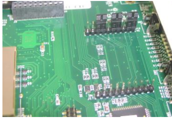
Figure 15: Jumpers across J16 installed
