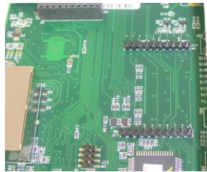
Figure 16: Jumpers across J16 removed
