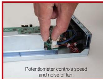
Potentiometer controls speed and noise of fan.
