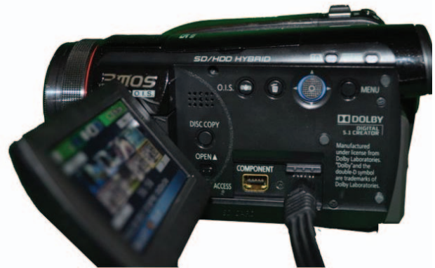
3.5mm connector plugged into the camera A/V output
