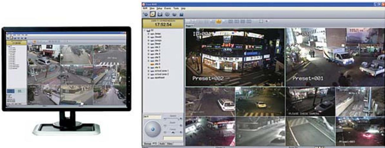
The TKC-100 is designed to work exclusively with the Marshall Video Management Software and does not work with the Live View in Internet Explorer. So even if you are using just one Camera you must have the VMS Software Installed.
