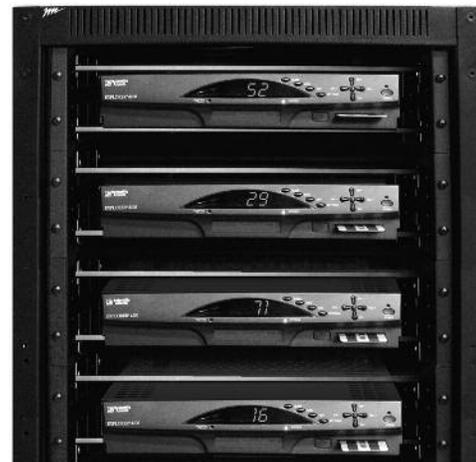
OCAP-3 (shown) uses three space model for greater heat dissipation, use two space model for high density mounting
