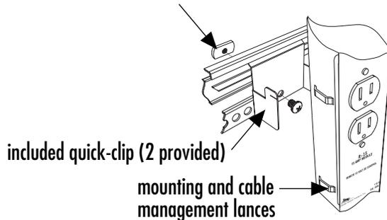
**NOTE:** Provided wood screws allow for mounting of mounting clip to wood surfaces
