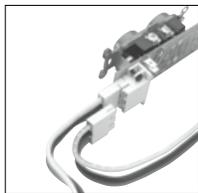
Interconnect modules with our unique genderless connectors - no hard wiring required!
