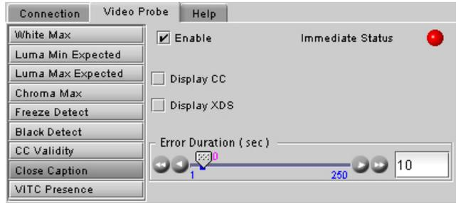
**VITC Presence:** Detects the presence of the input Time Code from a predetermined input line.
