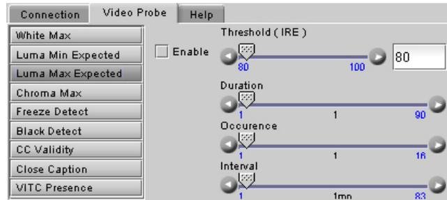
**Chroma Max:** Detects whether the amplitude of the chroma information in the video signal is too high by verifying if the peak chrominance of the input video signal is less than a specified threshold.
