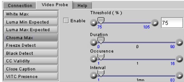
**Freeze Detection:** Detects whether a sequence of video frames are identical by verifying if it has been detected on the input signal, taking account of noise.
