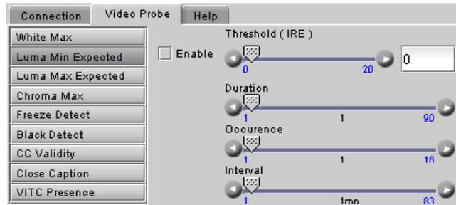
**Luma Max expected:** Detects whether the video signal contains some nearly-white information by verifying if the Luma component of the video signal includes information above a specified threshold.
