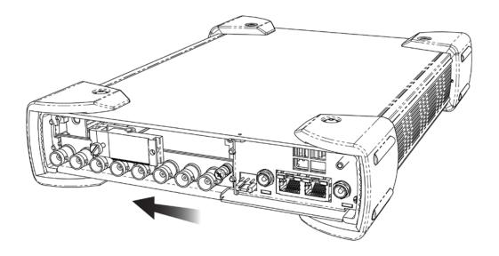
3. Finally, install the 2RU rear module – slip the left end of the 2RU rear module into the slot at the right end of the adapter, and secure it to the frame using the captive screw at the right end of the module.
