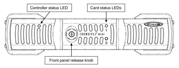
The card status LEDs and the controller status LED are visible on the front panel via light pipes as shown in the figure above.
