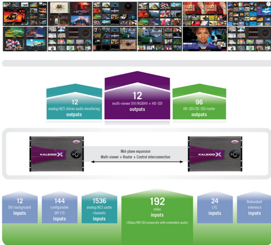
Kaleido-X (14RU) expansion system overview
