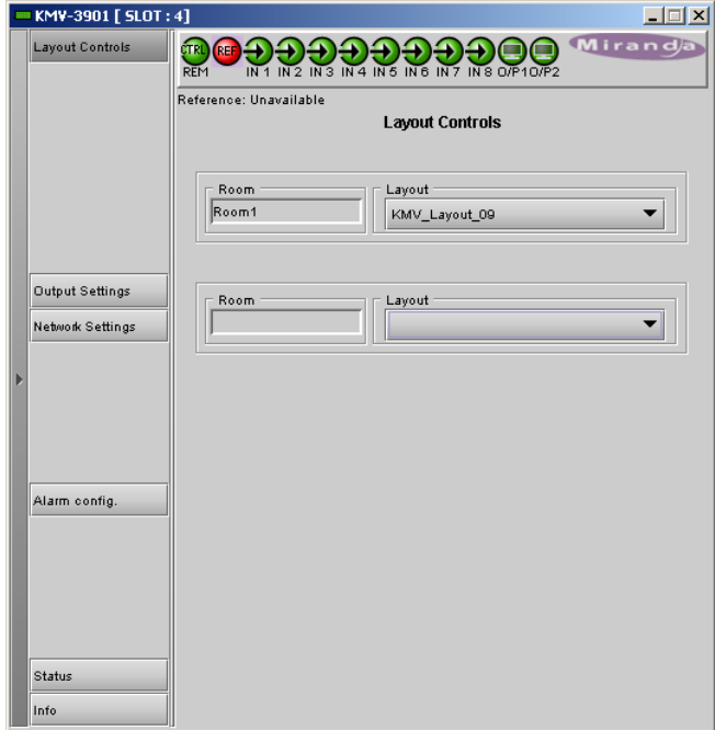
Figure 3.3 Layout Controls panel
