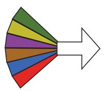
CWDM allows us to passively combine different wavelengths or "colors" of light without interference or crosstalk
