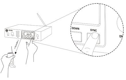
For syncing Receiver-Selected Frequency to Transmitter: Press the receiver Auto-Scan Button (29) to locate an open frequency/channel. Point the Receiver Infrared IR receptor/Sensor(22) at the transmitter Infrared Transmission Window (5) and press the SYNC Button (28) on the receiver until the transmitter's LCD Screen (4) displays the same frequency as the receiver's LCD Screen (21).
