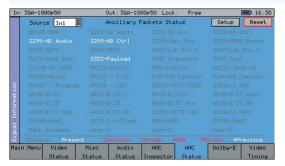
The Ancillary data status option provides a very quick status view of the ancillary data present in a SDI signal. It does not decode the data fully and is intended to be a fast analysis tool to show if a packet type is present, absent or red if in fault. Full logging is available along with DID and SDID custom setup.
