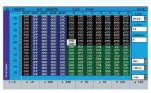
The **SDI** analysis option provides the engineer with a detailed view of the data words contained within the SDI stream. This allows the analysis of complex faults and is particularly useful when determining compatibility issues between equipment and when debugging new product developments particularly in a R&D environment.
