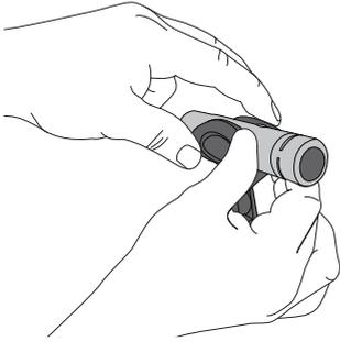
2. Grasping a clip in your left hand, attach it to one side of the stereo bar to the yoke by turning the screw on the stereo bar. Position the clip at a 45° angle to the stereo bar in the center of the mounting runner before completely tightening the screw.
