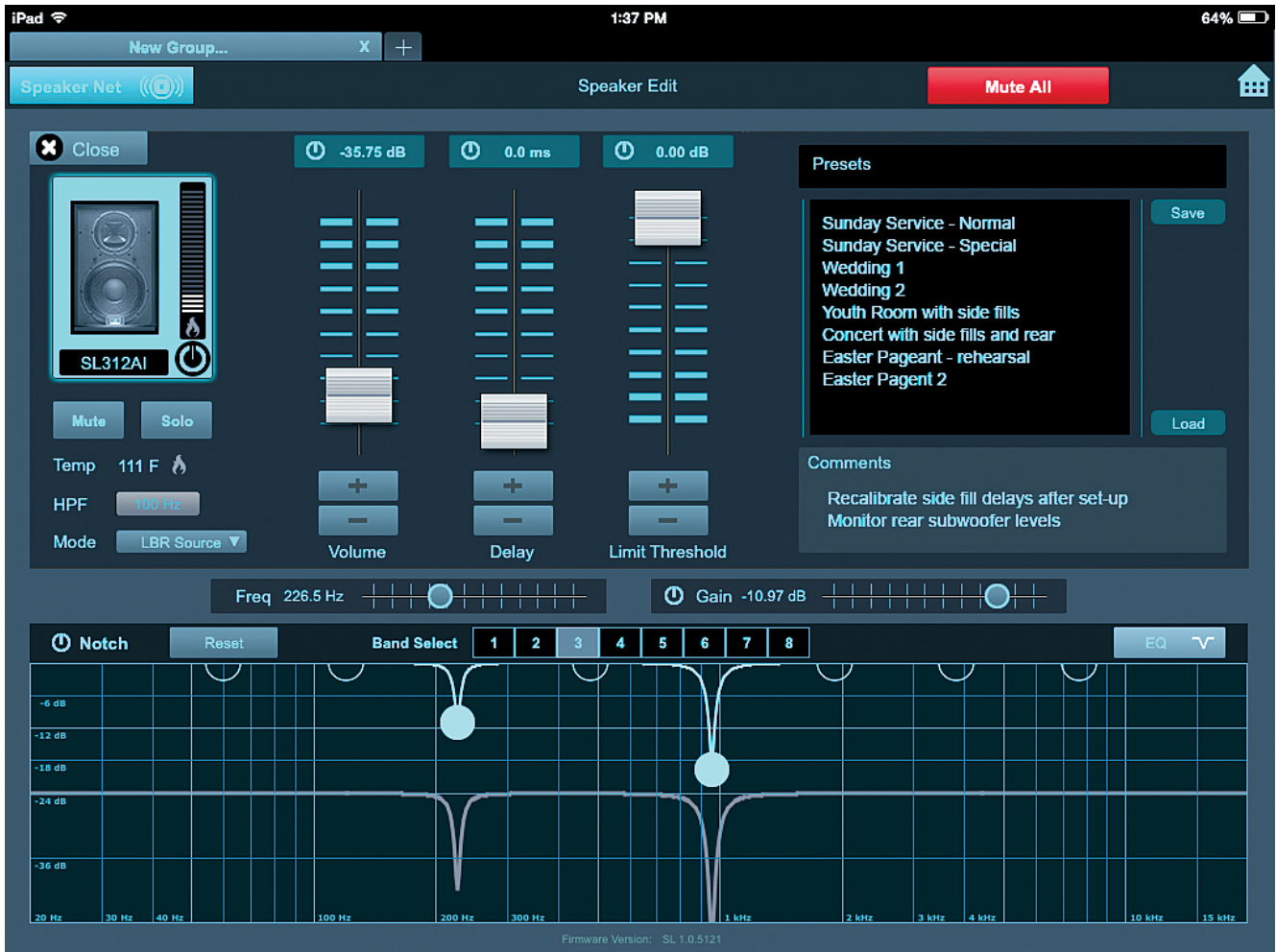
Speaker Edit page lets you set EQ, Alignment Delay, add Notch Filters, and remote control onboard speaker settings
