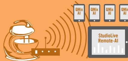
StudioLive AI-Series Mixers ship with both a USB WiFi LAN adapter and an onboard Ethernet connection. This lets you connect to a wireless router and wirelessly control your mixer from the
