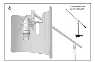
The VoxGuard may be used with a studio boom that features a down extension. Assembly is the same except the baffel and mic are inverted.
