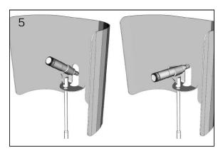
5. The VoxGuard is equipped with a rear access port for front address microphones. Use the rear port as an exit for the mic cable. This allows the microphone to be articulated over a wide range for precise positioning.
