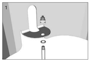
Begin by threading the knurled ring onto the microphone stand. If your stand already has a ring or flange you can use it instead. The knurled ring is intended for stands that do not have a ring or flange.
