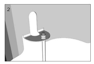
Slip the VoxGuard over the top of the microphone stand and secure it with the threaded adapter. The threaded adapter locks down the VoxGuard as well as provides the microphone clip a solid mount.
