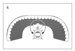
4. To center the mic, rotate the VoxGuard. It will move freely. Once in place, the VoxGuard will rest on the knurled ring. When you move the stand around it is normal that the VoxGuard will sway until it comes to the rest position.
