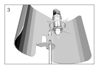
Once the ring and threaded adapter are installed you can screw on the microphone shockmount or clip. Changing mics does not require any disassembly. Simply remove one mic and replace with another.
