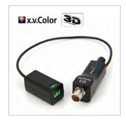
The EZ-S 3G/HD-SDI connector modules feature built-in electrical-to-optical conversion technology which extends the transmission distance without the need for additional components and repeaters. The compact balun simplifies installation even further and requires no adjustments, making setup quick and painless.
