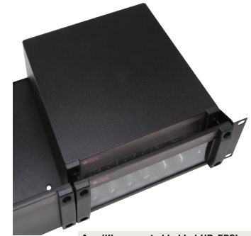
Amplifier mounted behind HD-FP2L
