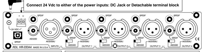
Connect one digital audio source to the appropriate input jack:
