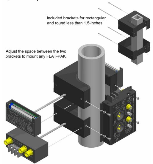
The PM-1V is designed to mount any RDL FLAT-PAK module to a projector pole. This is a vertical mounting system designed to grip a standard 1-1/2" I.D. pole common to most projector mounts. An included pair of bracket and screw sets allows mounting to poles smaller than 1-1/2" and to square or rectangular projector mounts. Adequate vertical pole clearance must be available for mounting the PM-1V. The bracket side plates are intended for the mounting of any RDL STICK-ON or TX series module.
