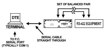
A PAIR OF RU-SC2S WILL ACT AS A NULL MODEM. USING A NULL MODEM CABLE WILL CAUSE THE SYSTEM TO ACT AS THOUGH THERE IS A STRAIGHT THROUGH CONNECTION.
