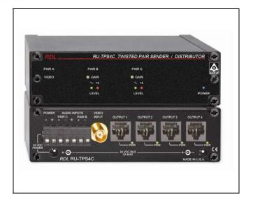
**APPLICATION:** The RU-TPS4C is a four output audio sender, video signal and power distributor module compatible with all RDL Format-C twisted pair products. A video source connects to the BNC input jack. Two line-level audio sources may be connected to the module using the +4 dBu balanced detachable terminal block. Studio-quality buffer amplifiers feed the three pairs of the four rear-panel RJ45 **OUTPUT** jacks at the correct operating level.
