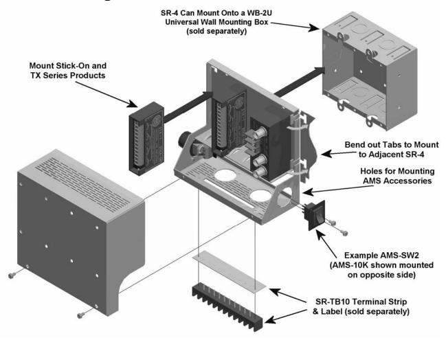
Mounting holes in the SR-4 permit attachment in a variety of locations, including cabinets, backboards, walls and plenums. The SR-4 holds up to 7 STICK-ONS. If power amplifier modules requiring convection cooling are mounted, a maximum of 4 should be installed, leaving an empty space between modules. 7 STICK-ONS may be mounted if they are not heat generating modules. TX<sup>™</sup> modules will also fit in the SR-4.
