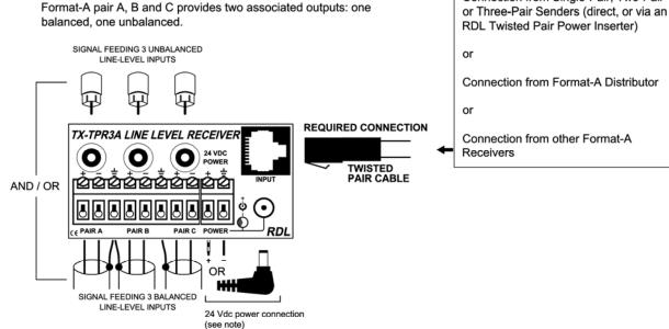
NOTE: Connect a 24 Vdc power supply to the module if power is not being supplied through a twisted pair cable from a connected module.
