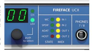
**Phones** is a low impedance line output of highest quality. It provides a sufficient and undistorted volume even when used with headphones.
