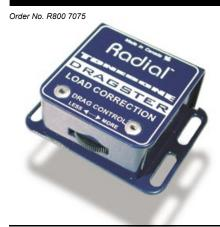
The Dragster is a load correction device designed to restore the full, rich tone you lose when you plug your guitar into a buffered input such as a wireless system. Dragster makes passive pickups "think" (and sound like) they're connected directly to an amplifier by simulating the impedance of an amplifier by allowing you to adjust the load on the pickup.
