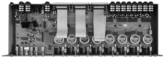
Shown in the default configuration with a direct line-level D-Sub output.
