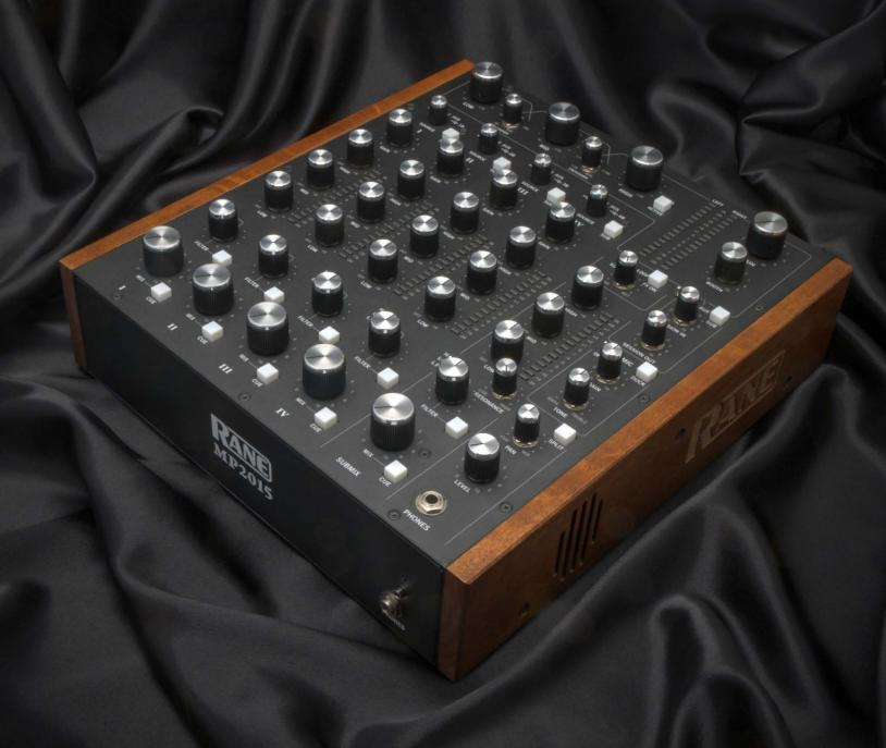
The MP2015 represents a perfect marriage of high-quality rotary control surface, state-of-the-art digital signal processing and dual 24-channel USB sound cards. This classy assortment of analog and digital I/O supports mixing vinyl, CD, S/PDIF and USB streaming audio content in any combination.
