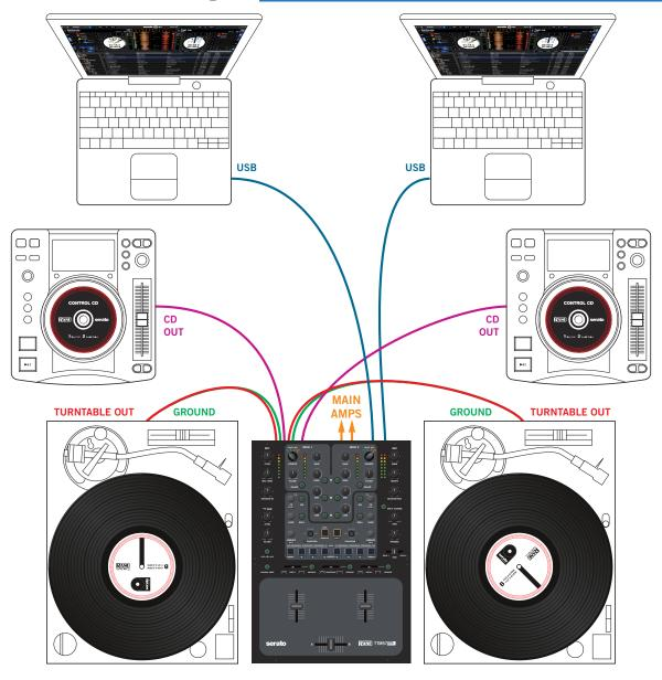
USB Port, x2 Each port can stream 20 channels of low-latency audio.
