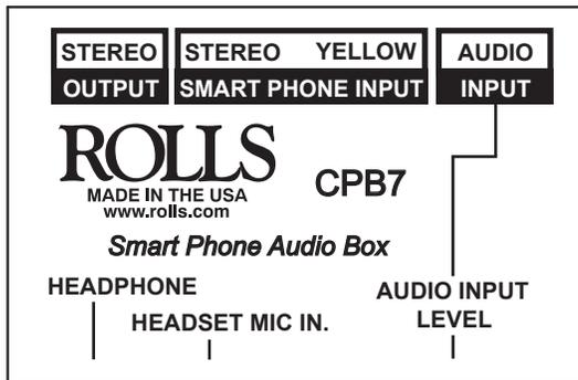
The CPB7 is a smart phone breakout box. It allows you to connect various inputs and outputs to your smart phone.
