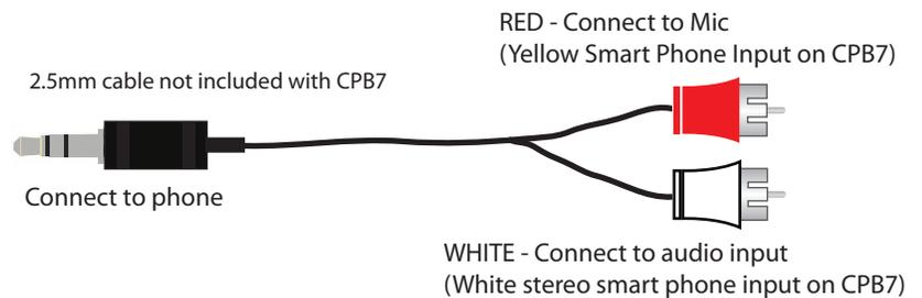
When using 2.5mm configuration you will only have mono operation for the audio section.
